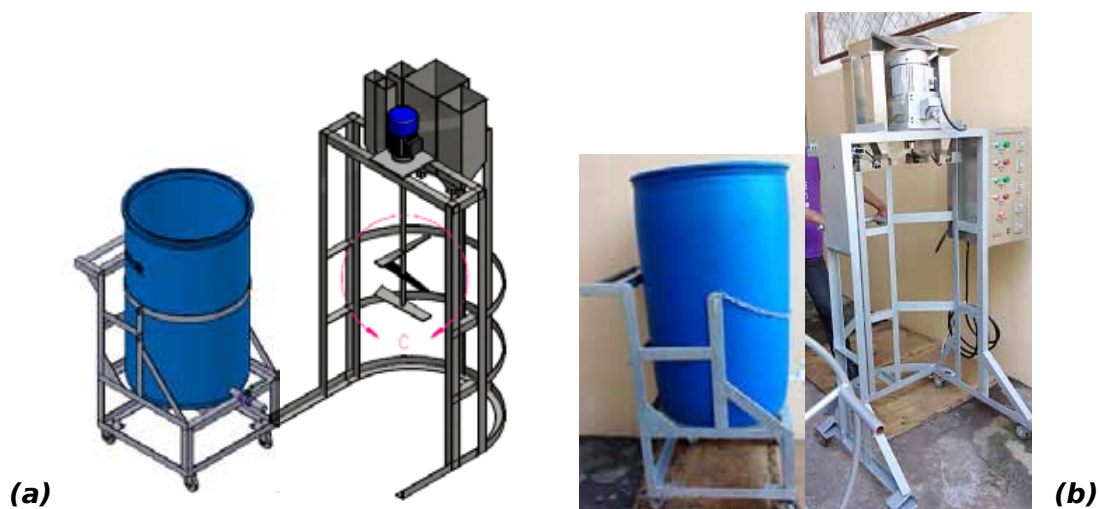
(a) Isometric view and (b) prototype unit of 100L reactor for liquid detergent/dishwashing
