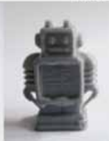
Printer: Ultimaker 2+ Material: PLA Build Plate Temp: 60C Nozzle Temp: 210 C
