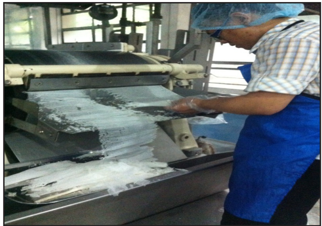
Production of drum-dried mango and makapuno at the FPD Pilot Plant.
