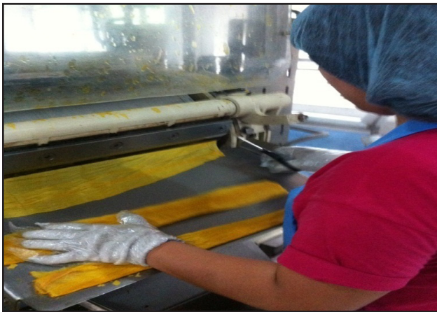
Production of drum-dried mango and makapuno at the FPD Pilot Plant.
