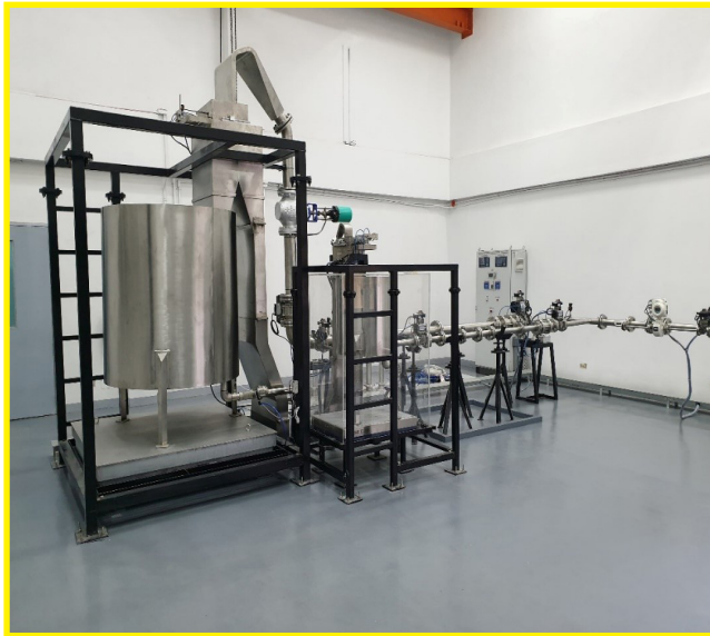
120 L and 1 200 L Collection Tanks mounted on weighing scales.
