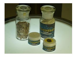
in polymer nanocomposites to improve their mechanical strength, toughness, electrical or thermal conductivity. In turn, the nanocomposites produced with nanoclay find application in making various commodity and engineering products for the automotive, construction, electronics, and packaging industry.
