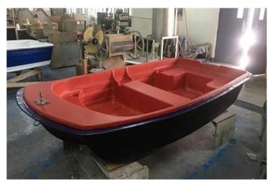
assisted resin transfer molding (VARTM) or resin infusion process, an innovative technique in fabricating abaca fiber-reinforced composites in more complex structures for different transport modes such as tricycle roof, fuselage for drones, and boat body.
