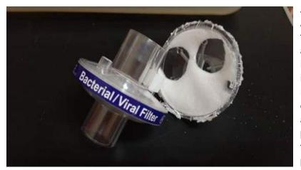
According to Dr. Meyvell G. Atanoso, the UST Hospital typically uses bacterial/viral filter, also known as a Heat and Moisture Exchange (HME) filter, ventilators in their and respirators. However. the difficulty of acquiring HME filters amidst this health crisis has prompted the hospital to search for an alternative filter that performs similarly to HME filters.
